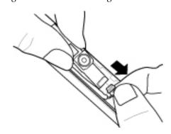
Figure 4-50 Disconnecting the CCD cable
